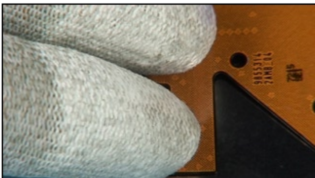
25. Smooth down the TOP FLEX ASSEMBLY evenly.
